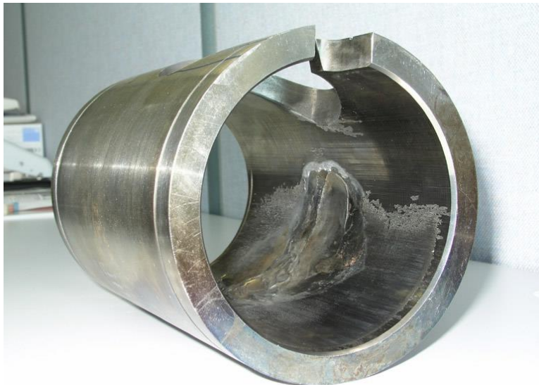
Worn inset after few thousand cycles
